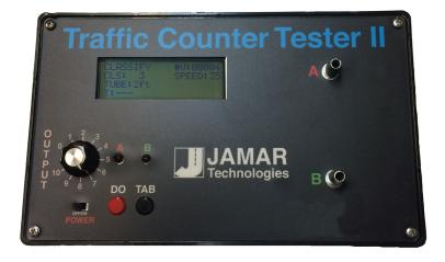
There are two push-button switches located at the bottom of the front panel. These buttons, labeled TAB and DO, are used to step through each operating mode, as well as to activate a mode. There are two LEDs located above the switches, labelled A and B. These LEDs correspond to the output nozzles, and give a visual indication of the air pulse. To the left of the LEDs is the Output dial. This dial controls the intensity of the air pulses generated by the TCTII.
